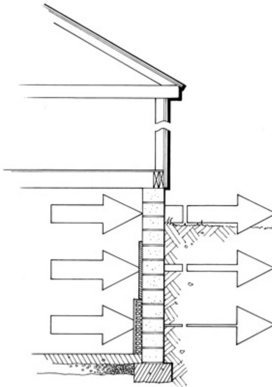
The calculations below assume a 20' x 30' [6m x 9m] basement with 2' [.6m] above grade and uniform 8" [20 cm] concrete walls. Doors or windows in poorly insulated homes would generally make the heat loss calculations worse. The calculations are averaged to take into consideration the fact that outside temperatures are warmer below grade.
